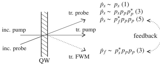
**Figure 1** Illustration of the investigated pump–probe setup, including incoming and transmitted light pulses (reflected pulses are omitted for clarity) for probe, pump, and FWM direction (the angle between the different propagation directions is strongly exaggerated). Selected contributions to the probe and FWM polarizations are schematically included in the figure. The numbers in parentheses indicate the lowest order in the external fields in which they appear.
